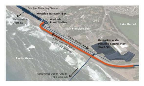
Sewer Piping diagram and Pumping Plant (above)
