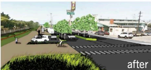
Figure V-4b: Proposed Sloat Blvd = Bike Lane + Pedestrian Walk + Diagonal Parking Pockets + 2 Driving Lanes + Planted Median + 2 Driving Lanes
